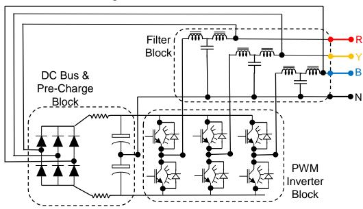
As can be seen from the diagram, the power section block is mainly made up of three broad blocks.
